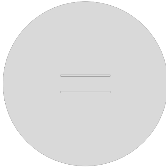
Fig. 2. Parallel plate capacitor model surrounded by a circular area within which we will perform the calculations.
